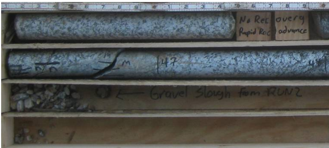
BV-4P close up of gravel slough. Gravel is likely from zone of no recovery.
